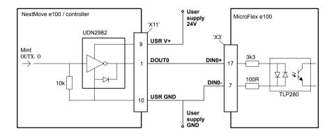
Figure 27 - Digital input - typical connection from a Baldor NextMove e100
